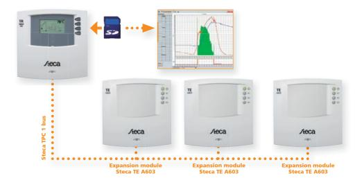
Example of application 2: System controller Steca TR 0603mc with the heating controller Steca TH A603 MS and the expansion module Steca TE A603
