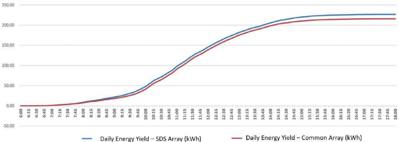
Figure 3-23 Comparison of the accumulated energy yields of inverters between SDS arrays and common arrays
