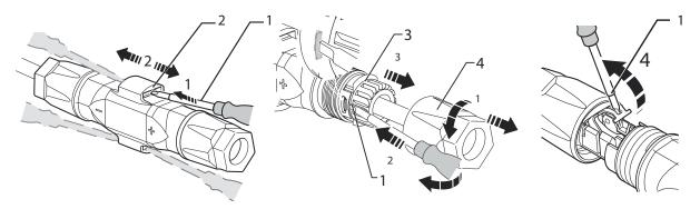
Figure 43: Disconnect connector
