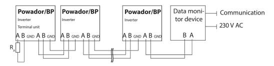
Figure 32: RS485 interface wiring diagram
