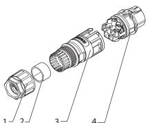
Figure 15: AC connection plug
