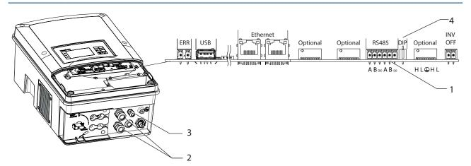
Figure 31: Connection area: Connection and assignment of the interfaces
