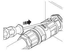
Figure 40: Disconnect the AC connection plug from the device connector
