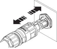
Figure 41: Disconnect AC connection plug
