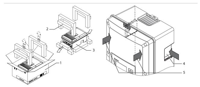
Figure 8: Unpacking the unit
