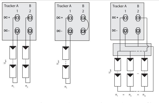
Figure 26: Two generators each on oneFigure 27: One generator on 1st tracker,Figure 28: One generator parallel onMPP trackersecond tracker eactivatedboth MPP trackers
