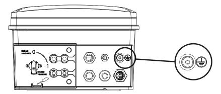
Figure 29: Grounding point in the connection area
