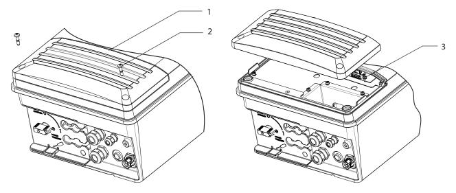
Figure 30: Access to connection area of the interfaces
