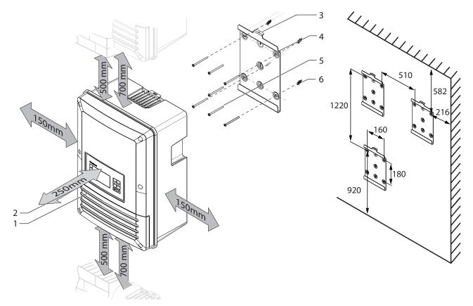
Figure 10: Minimum distances/wall bracket
