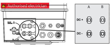
Figure 25: Connections for DC positive and DC negative
