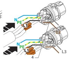
Figure 17: Connect cable to the contact carrier
