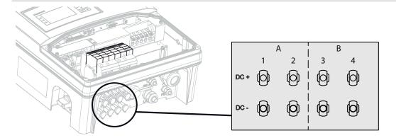
Figure 18: Connections for DC positive and DC negative
