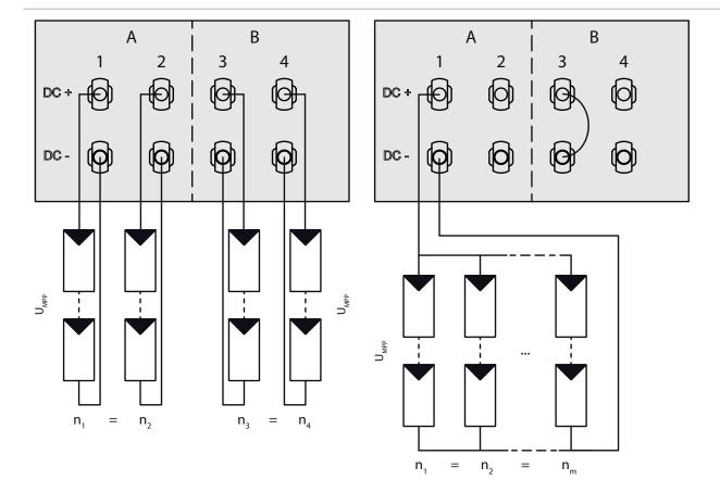
Figure 19: Recommended standard connection
