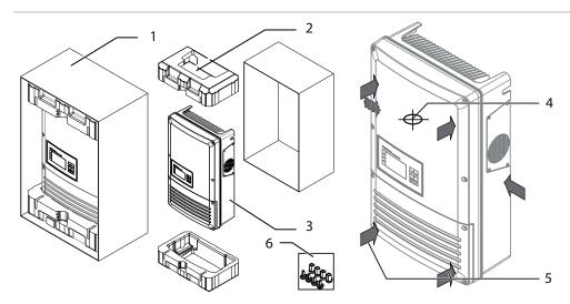
Figure 8: Unpack the inverter
