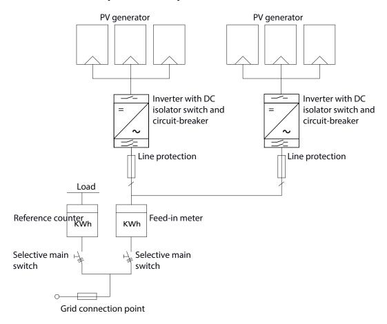
Figure 4: Circuit diagram of a system with two inverters
