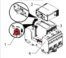
Figure 33: DC overvoltage protection
