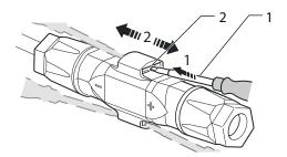
Figure 34: Disconnect connector
