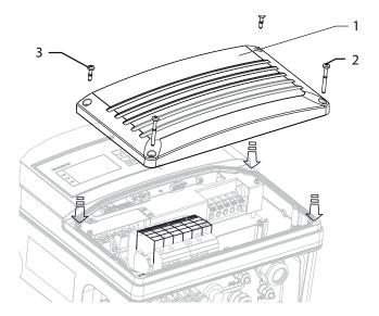
Figure 12: Connection area: Open connection cover
