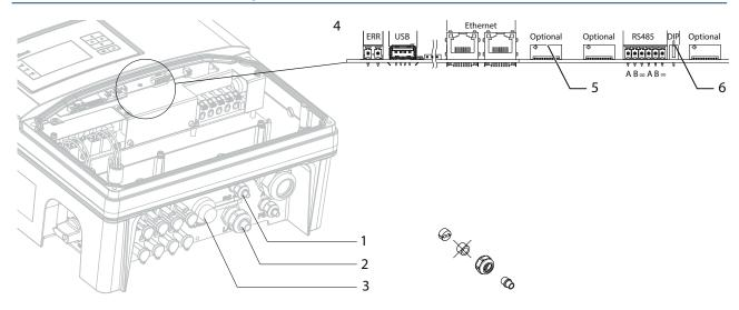
Figure 22: Connection area: Connection and assignment of the interfaces
