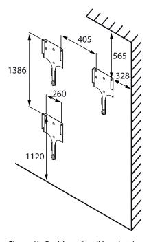
Figure 10: Minimum distances/wall bracket
