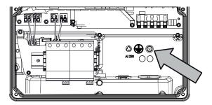
Figure 21: Grounding point in the connection area
