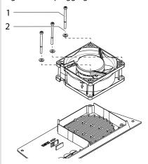
Figure 31: Mounting the fan
