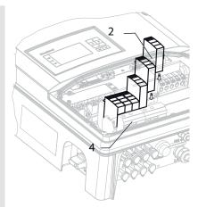
Figure 32: Install surge protection device modules
