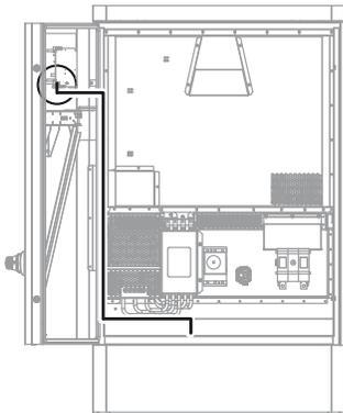
Figure 17: Routing the interface cable
