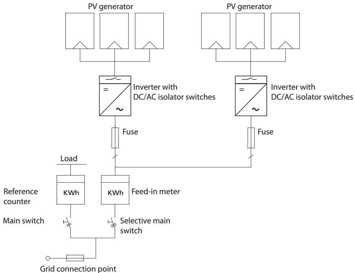
Figure 1: Circuit diagram of a system with two inverters
