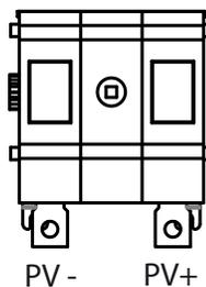
Figure 13: PV connection (M1)
