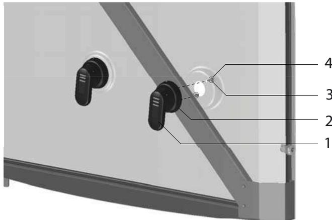
Figure 8: Installing the DC and AC isolator switches
