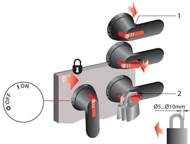
Figure 3: DC/AC isolator switches
