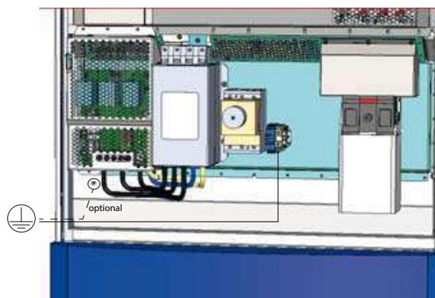
Figure 15: Grounding point in the connection area
