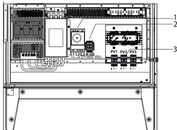
Figure 11: Electrical connection (M3 Model)
