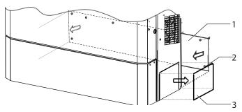
Figure 13: Perforation on the housing base /rear plinth panel
