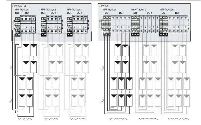
Figure 26: Recommended standard connection, XL variant (left: 39.0 TL3, right: 72.0 TL3)
