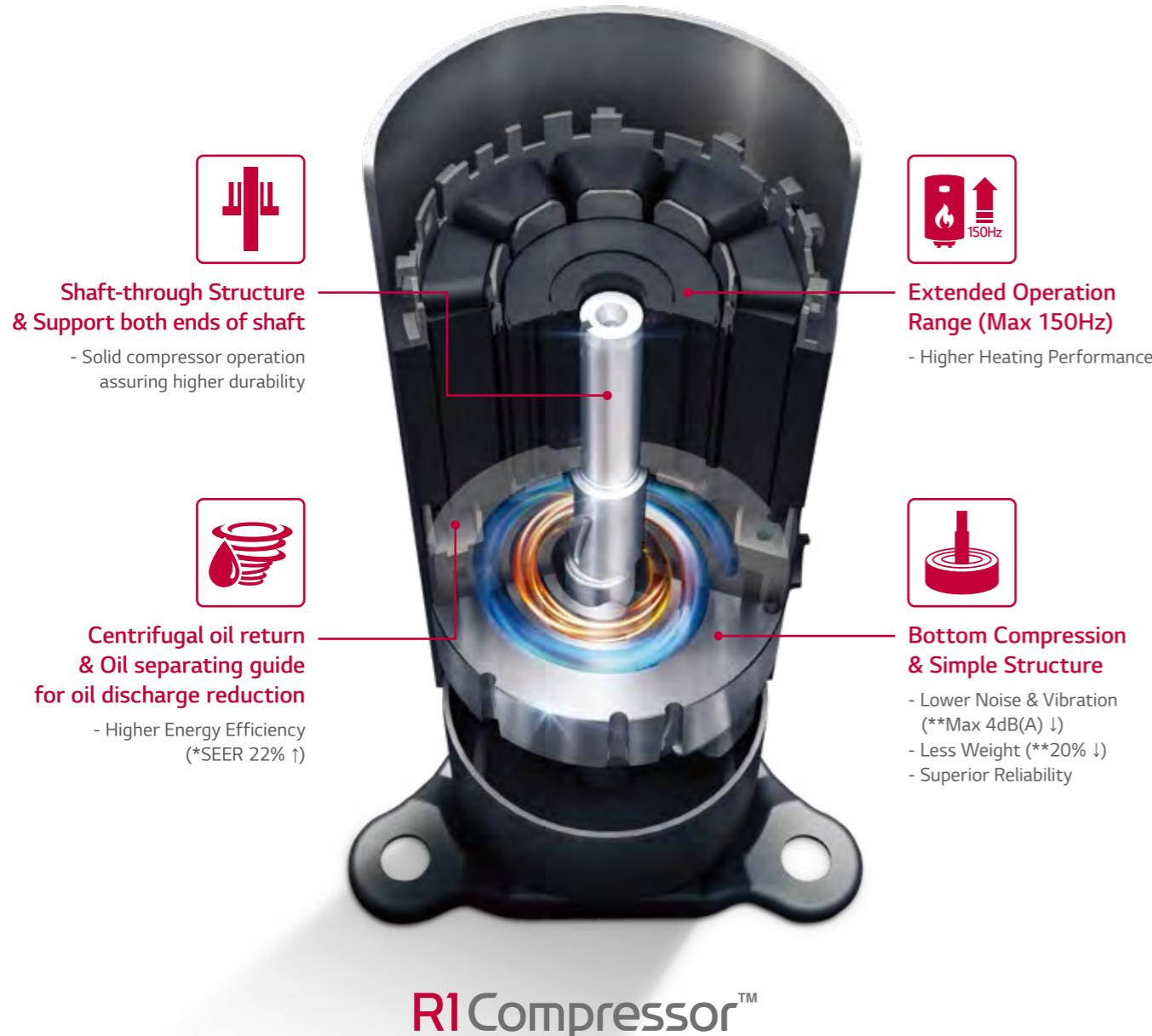
\* LG Internal test result, Based on single split 10 kW Cassette
