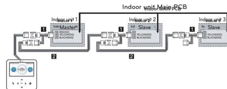
① Group control cable (PZCWRCG3): Connect to indoor unit's wired remote controller connector
