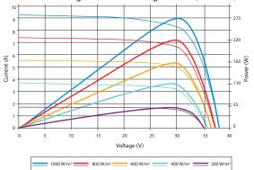
Excellent performance under weak light conditions: at an irradiation intensity of 200 W/m² (AM 1.5, 25 °C), 95.5% or higher of the STC efficiency (1000 W/m²) is achieved
