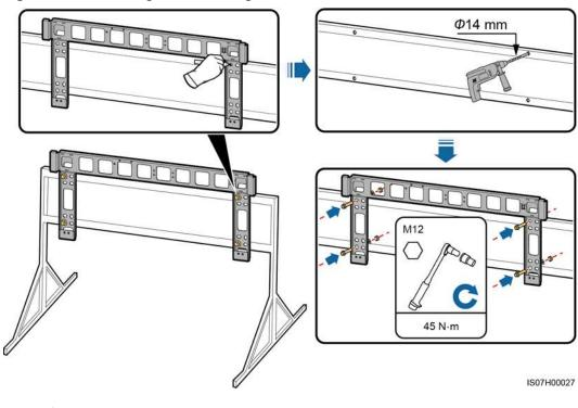
Figure 4-10 Installing the mounting bracket
