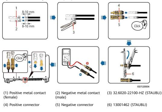
Figure 5-13 Installing the DC input power cable (MC4 EVO2 PV Connectors)
