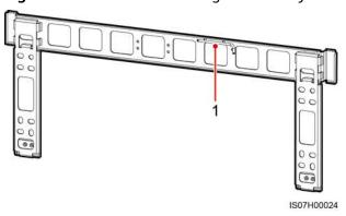
(1) Position for binding the security Torx wrench
