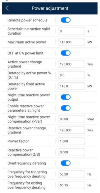
**Figure 7-13** Power adjustment parameters
