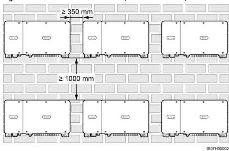
Figure 4-7 Stacked installation mode (not recommended)
