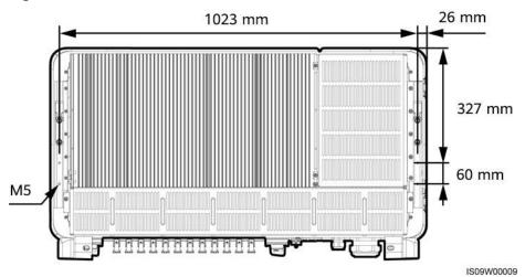
Four M5 screw holes are reserved on the rear of the SUN2000 for installing an awning.
