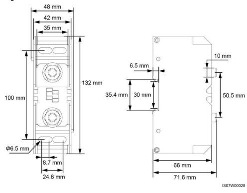
Figure 5-9 AC terminal block dimensions
