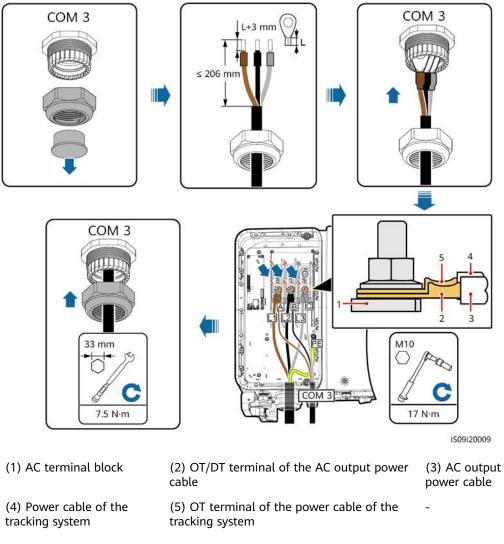
Figure 5-17 Connecting the power cable of the tracking system
