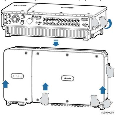
Figure 4-14 Lifting the SUN2000 and keeping it upright
