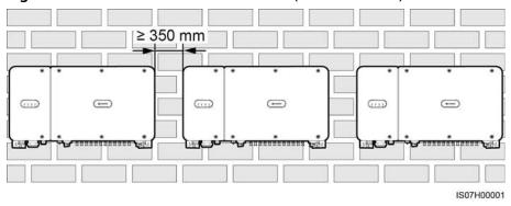
Figure 4-6 Staggered installation mode (recommended)
