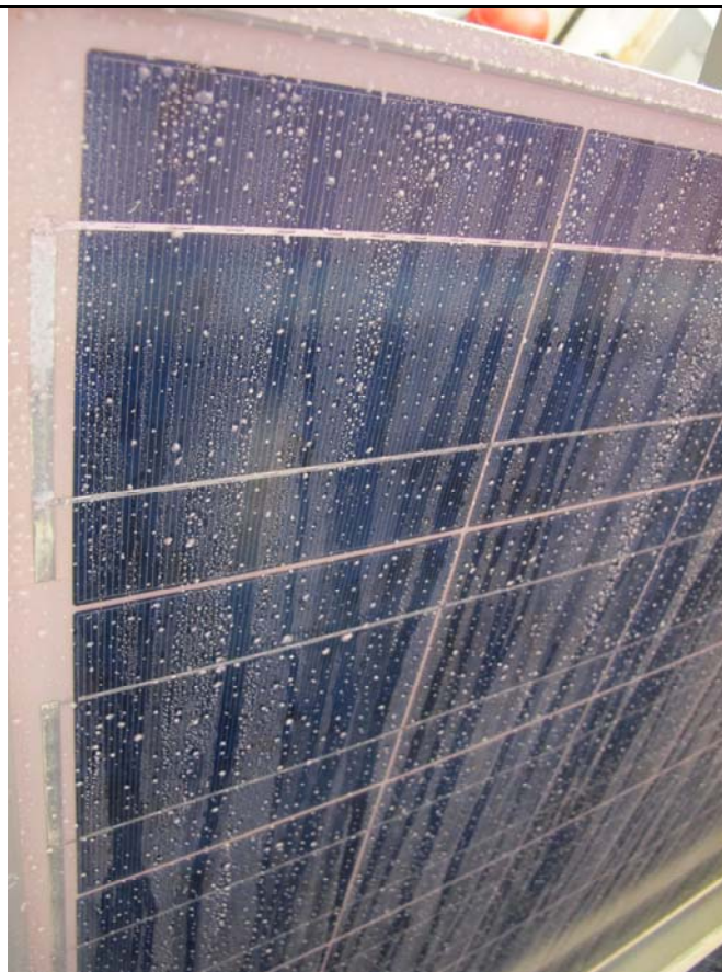
Photo 6 sample after salt mist test: strong salt deposit at the surface (before cleaning process)
