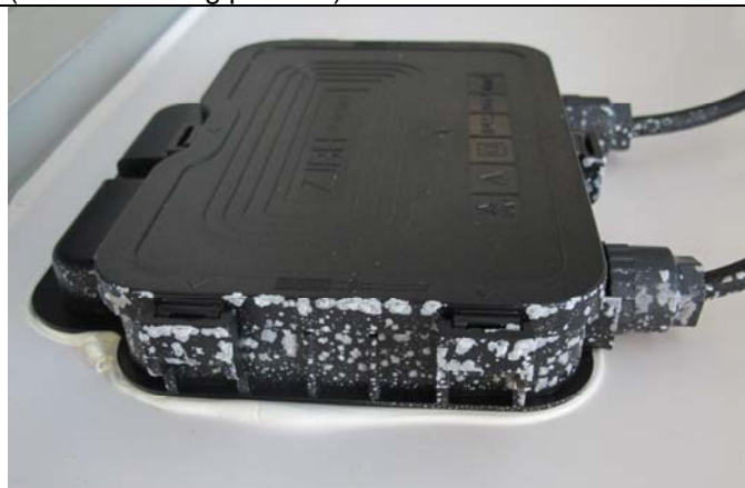
Photo 8 sample after salt mist test: Electronic case with salt deposit on the surface. The case has not been opened.
