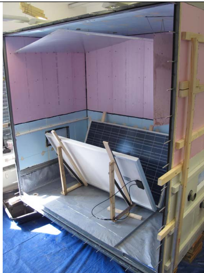
Photo 3 sample (initial state) inside the 8m³ test chamber The connector are closed, angle 30° from vertical
