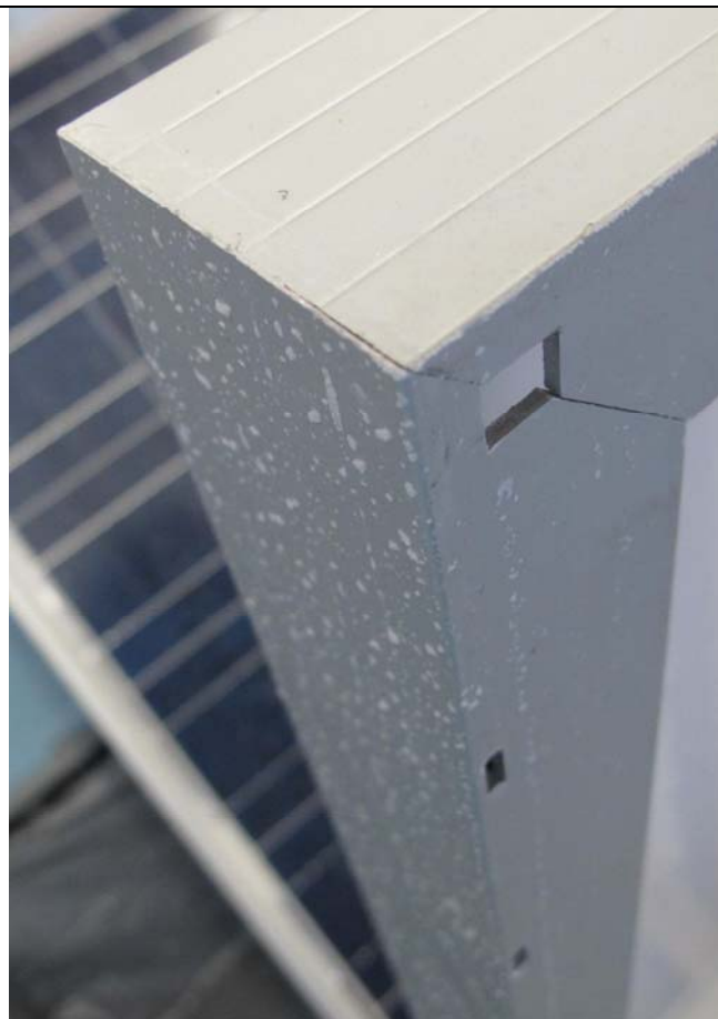
Photo 7 sample after salt mist test: The aluminium frame show no corrosion on the surface, etch and corner.
