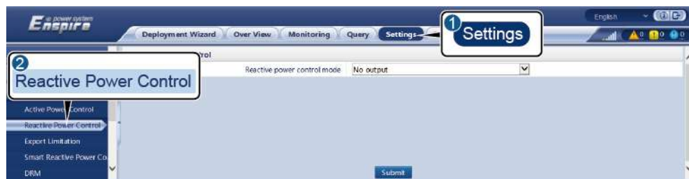
Figure 6-43 Reactive power control
