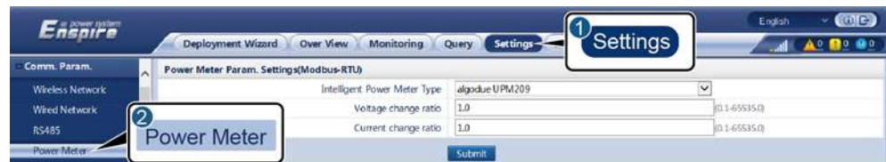
Figure 6-24 Setting power meter parameters
