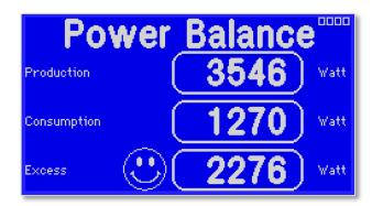
If a meter reader in the Solar-Log<sup>1000</sup> is configured with the "consumption meter" model, an additional "Power balance" dialogue box is available on the touchscreen. In this dialogue box, the current power values are shown and the surplus power is calculated. Depending on the surplus amount, a "smiley" indicates whether it makes sense or not to switch on consumers manually at that moment.
