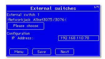
Depending on the switch model selected, various additional addresses must be entered, e.g., the IP address for the network outlet. Please note that the IP addresses of the outlets must be positioned in the same address area in which the Solar-Log<sup>TM</sup> is also located. To set the IP address for the network outlet, please read the accompanying manual or ask a network expert.
