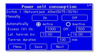
After defining the switches, the controls must be configured. These settings are made in the dialogue box "Analysis / Self consumption".
