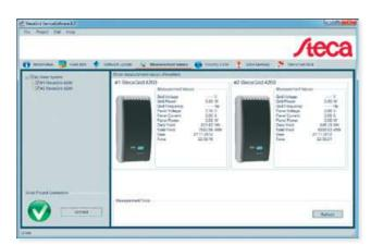
Current measured values of the StecaGrid inverters connected to the RS485 bus
