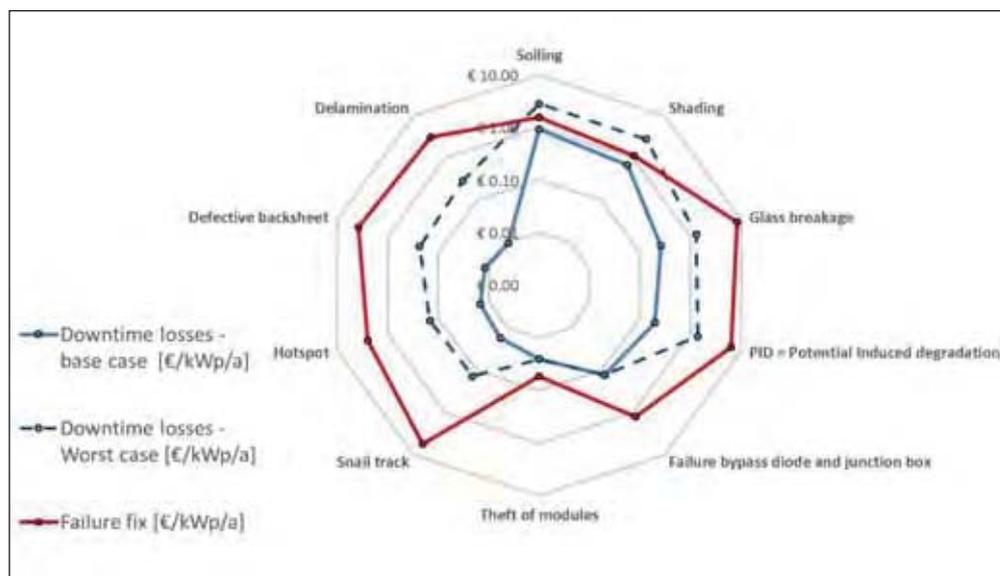
**Figure 3. CPN values resulting from the statistical analysis for the top ten technical risks for PV modules. The red line represents the cost/kWp/year of fixing the specific failure. The dashed and solid blue lines represent the cost/kWp/year due to downtime in the worst and base case scenarios respectively**
