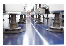
Fig. 2: Load testing at the Hanwha Q CELLS test center.
