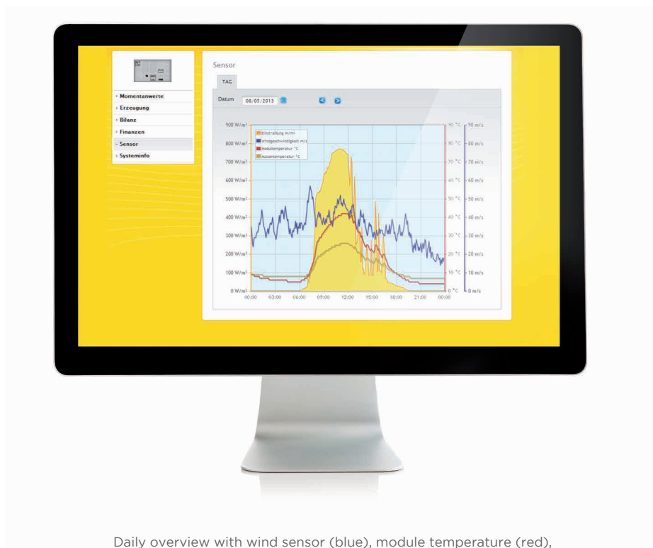
Daily overview with wind sensor (blue), module temperature (red), ambient temperature (green) and yield curve (yellow).
